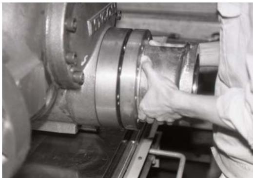
Photo 017 Removing High-stage Unloader Cylinder
