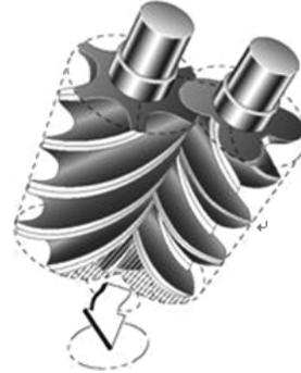
Figure 2-13 Discharge Process
