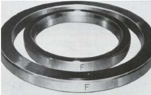
Photo 048 Stamp Marks on Spacer (Outer) and Alignment Spacer (Inner)
