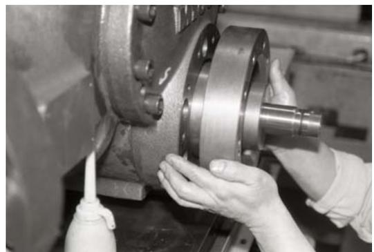
Photo 018 Removing Cylinder Guide B
