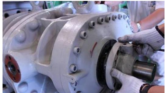
Photo 022 Removing Seal Cover
