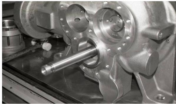
Photo 029 Unloader Cylinder Guide A
