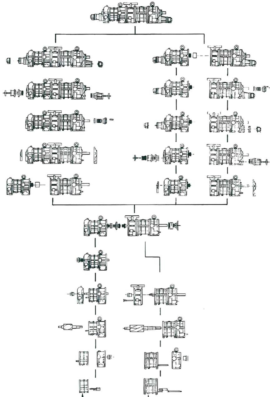
Figure 5-1 Illustrated Disassembly Sequence
