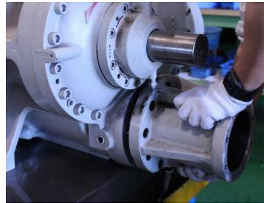
Photo 016 Removing Low-stage Unloader Cylinder
