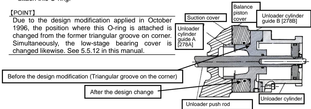
Figure 5-21 Modification of O-ring Attaching Position
