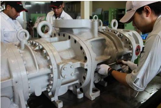
Photo 030 Tapping Alignment Pin
