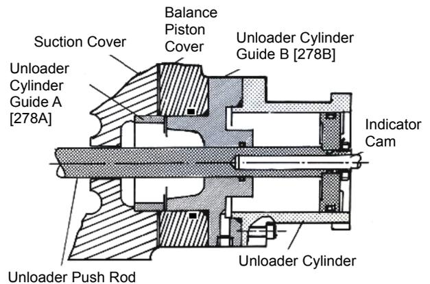
Figure 5-8 Unloader Cylinder Block (High-stage)
