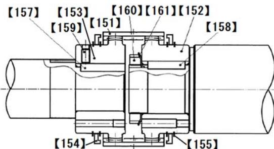
Gear coupling assembly comprising 151, 152, 153, 154\*2, 155\*2 and 159.
