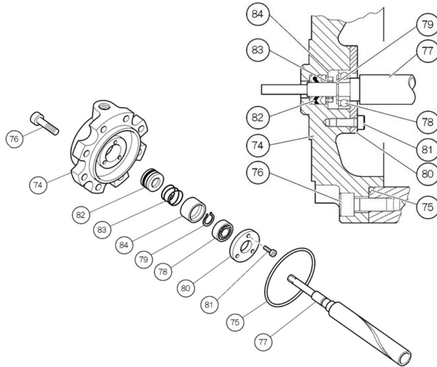
**Figure 5-24 Unloader Cover Block**
