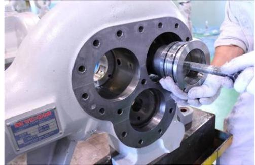
Photo 042 Removing Side Bearing
