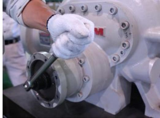
Photo 015 Loosening with Lock Nut Wrench
