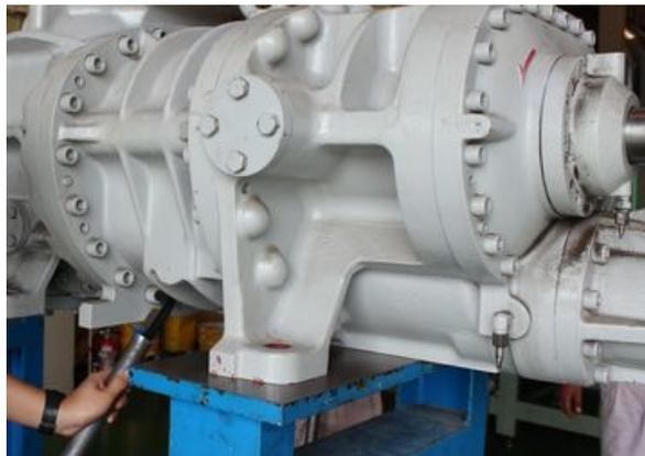
Photo 003 Loosening Lower Flange Fastening Bolts
