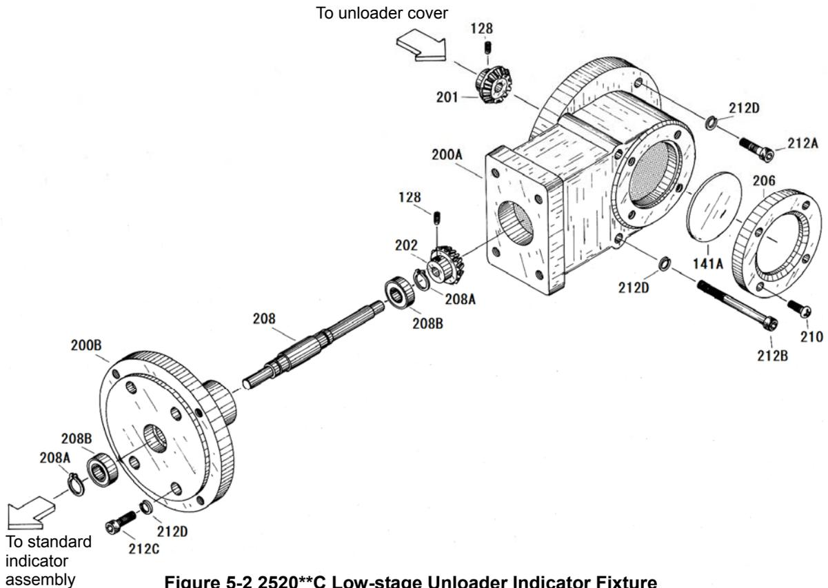
Figure 5-2 2520\*\*C Low-stage Unloader Indicator Fixture
