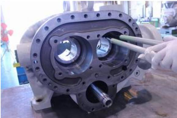
Photo 060 Removing Snap ring
