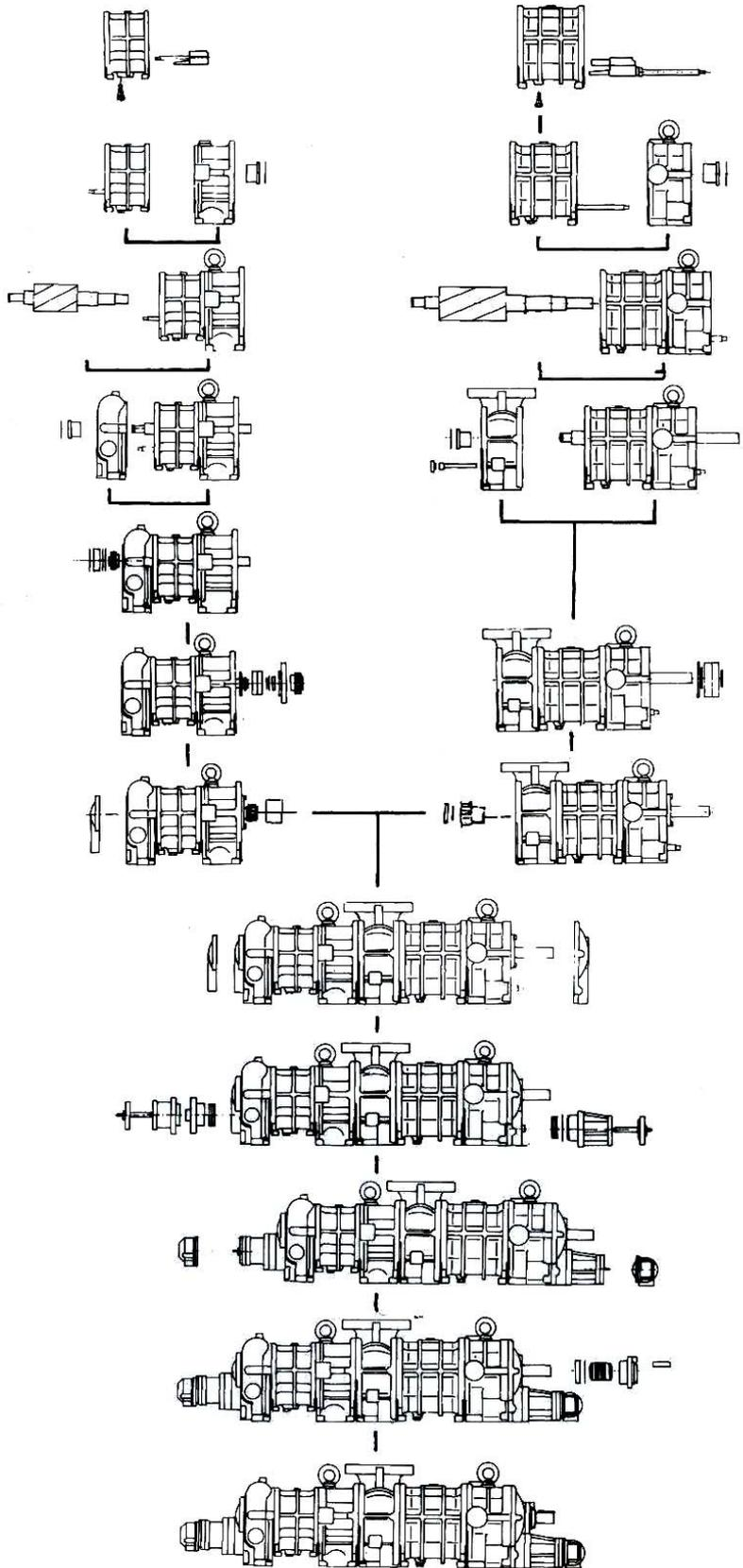
Figure 5-16 Illustrated Assembly Sequence (Example)
