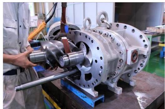
Photo 070 Attaching F rotor
