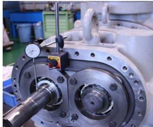
**Photo 098 Measurement of Runout**
