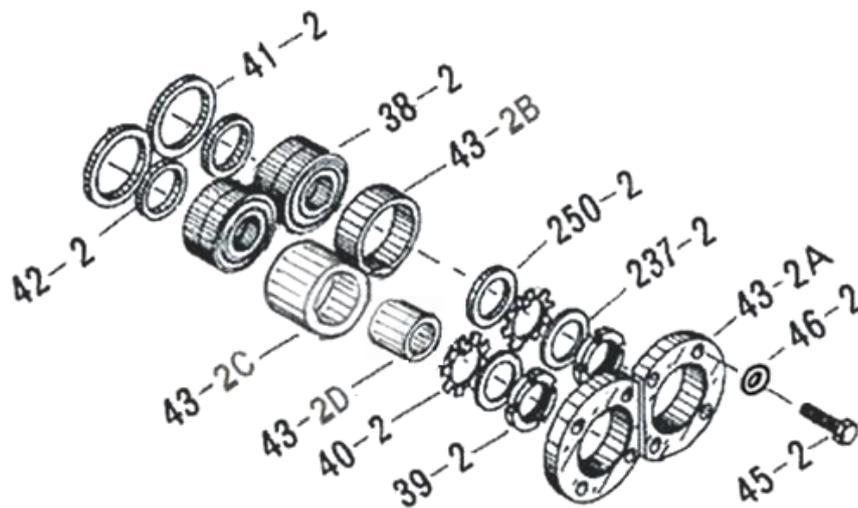
Figure 5-13 High-stage Thrust Bearing Block
