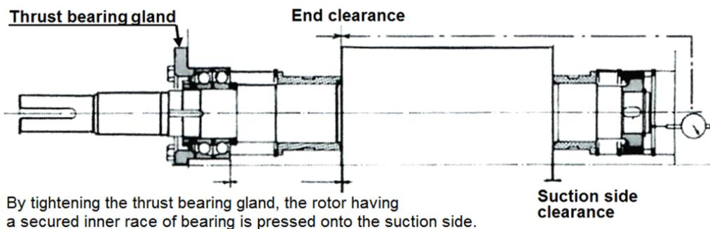
**Figure 5-20 End Clearance Measurement**
