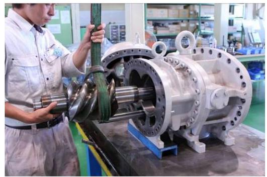
Photo 053 Lifting up M Rotor
