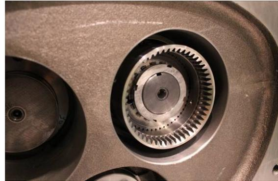
Photo 033 Low-stage Gear Coupling
