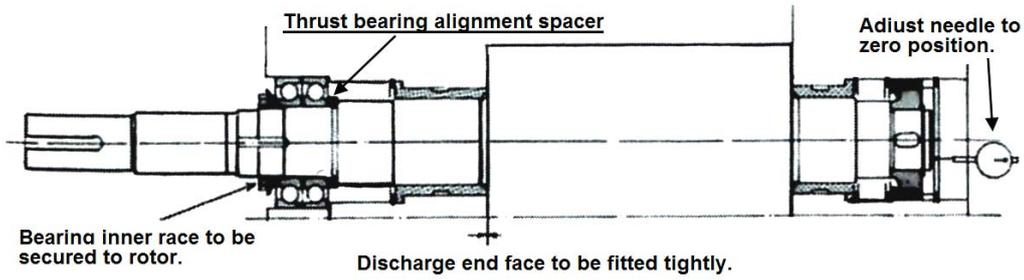
**Figure 5-19 End Clearance Measurement Preparation**
