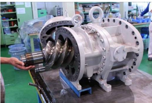
Photo 052 Pulling out M Rotor
