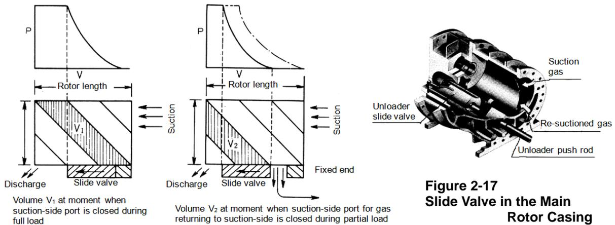
Figure 2-16 Capacity Control Mechanism
