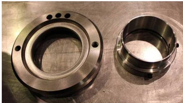
Photo 025 Oil Seal Retainer and Oil Seal Sleeve attached with O-ring
