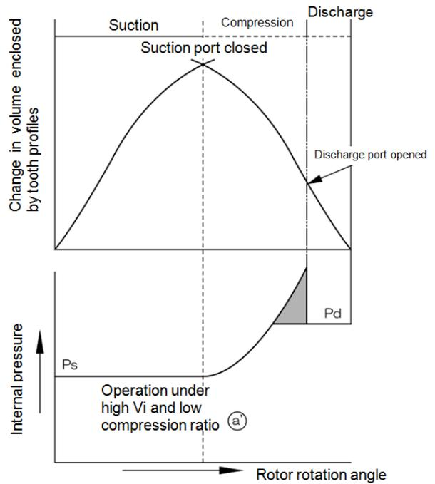
Figure 2-15 Relationship between Volume Ratio ( $V_i$ ) and Operation Conditions
