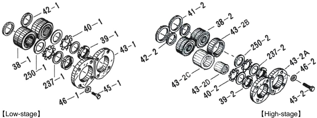
Figure 5-18 Thrust Bearing Block
