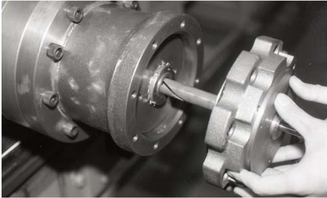
Photo 010 Pulling Out Unloader Cover
