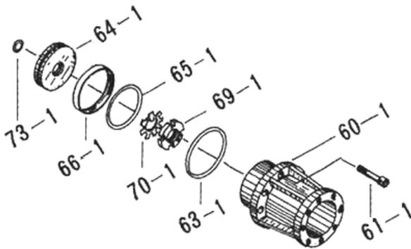
Figure 5-5 Unloader Cylinder Block (Low-stage)
