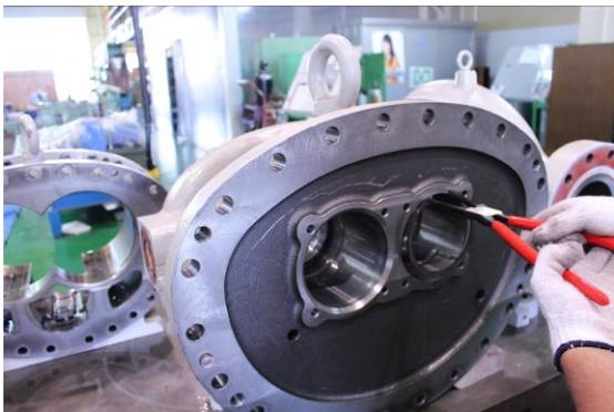
Photo 058 Removing Snap ring
