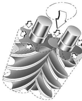
Figure 2-10 Compressor Mechanism
