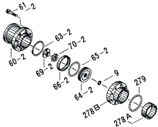
Figure 5-6 Unloader Cylinder Block (High-stage)
