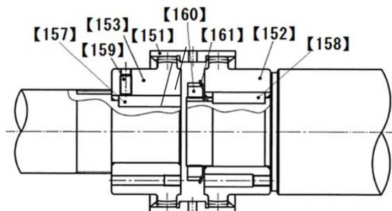
Gear coupling assembly comprising 151, 152, 153 and 159.
