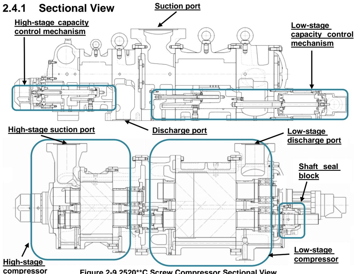
Figure 2-9 2520\*\*C Screw Compressor Sectional View
