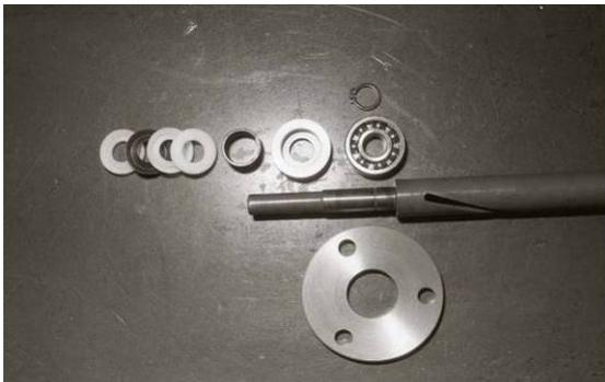
Photo 012 Parts Attached to Indicator Cam
