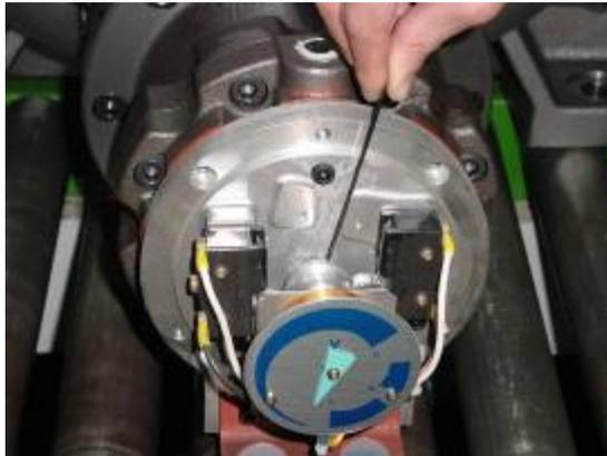
**Loosen the Set Screw of the Micro Switch Cam**
