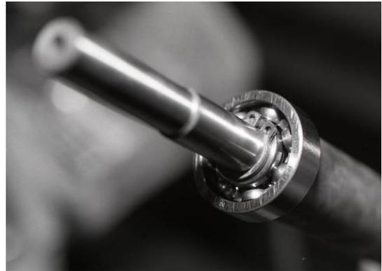
Ball Bearing for the Indicator Cam
