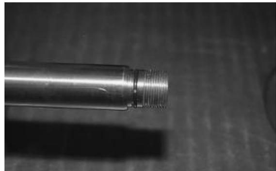
O-ring [63] at the tip of Unloader Push Rod
