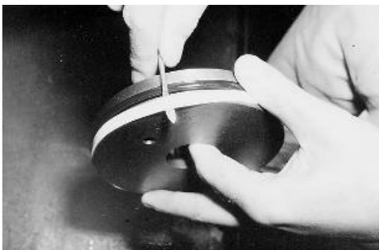
Removing the Cap Seal
