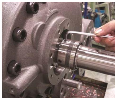
Loosen the set screw of the seal collar
