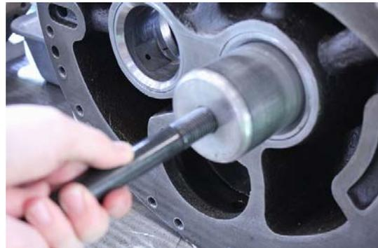
Installing the Bearing using the Jig
