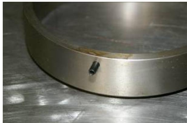
Type 2: Locked by a Spring Pin
