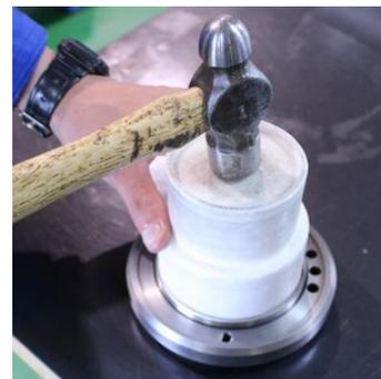
Using a Teflon block or the like as a pad (right above picture), lightly hit the pad to push the oil seal evenly into the retainer until it is fully seated. Once the oil seal is fully inserted, you can easily sense it as the hitting sound as well as the response will change.
