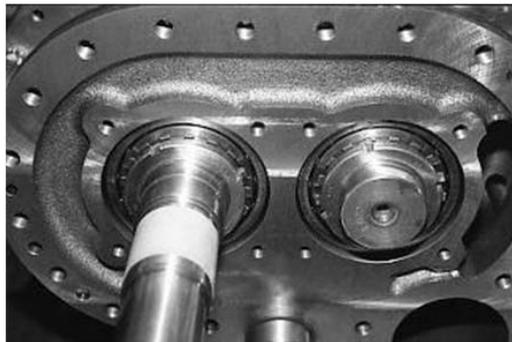
After tightening the Lock Nut
