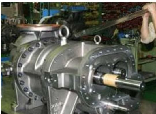
Tightening the Bolts using a Torque Wrench
