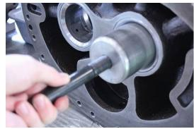
Aligning the Bearing position using Guide Bar
