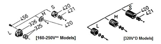
, Figure 5-9 Unloader Piston Spacer and O-rings
