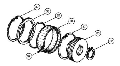
Figure 5-10 Exploded View of Balance Piston Block
