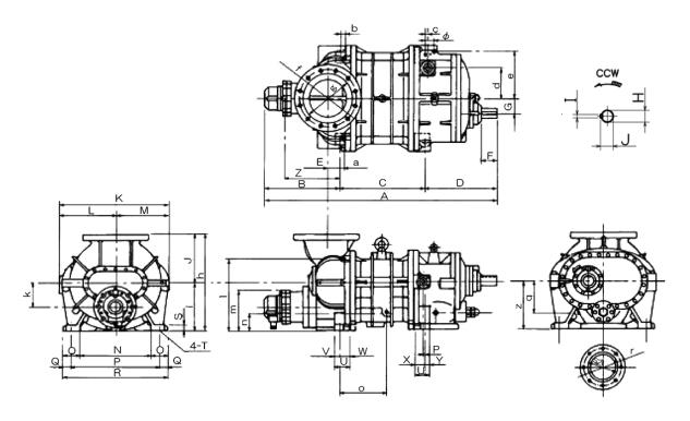
Figure 2-2 Outer Dimensions 160V\*G, 200V\*G, 250V\*G, 250VLLG (Down discharge type)
