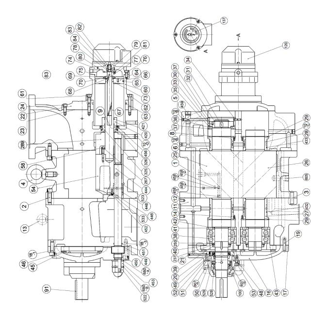
Figure 7-4 Sectional View (160 to 250V\*G model)
