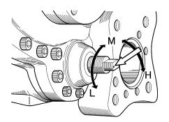
Figure 4-1 Vi Adjusting Rod
