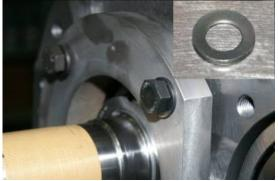
Removing the Thrust Bearing Gland
