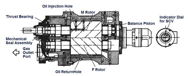
Figure 2-4 Compressor Structure (Representative View of Sideways Discharge Type)
