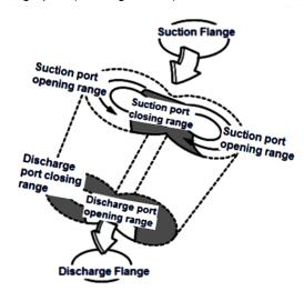
Figure 2-5 Suction and Discharge Port
