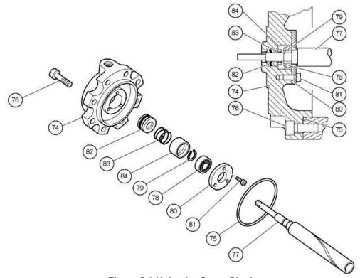
Figure 5-6 Unloader Cover Block
