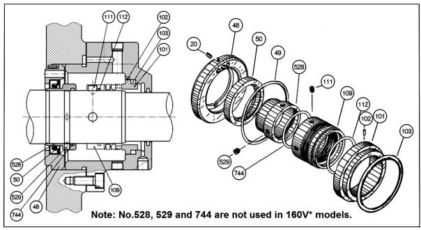
Figure 5-19 BBSE type Mechanical Seal Assembly and Related Parts
