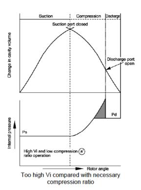
Figure 2-13 Proper and Improper Adaptation of Vi to Load Condition
