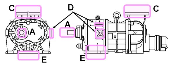
Figure 1-2 Hazardous Sources (Compressor: V\*G type i.e. discharge port facing down)
