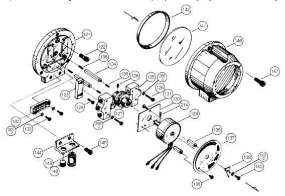
Figure 5-4 Traditional Standard type Unloader Indicator Assembly
