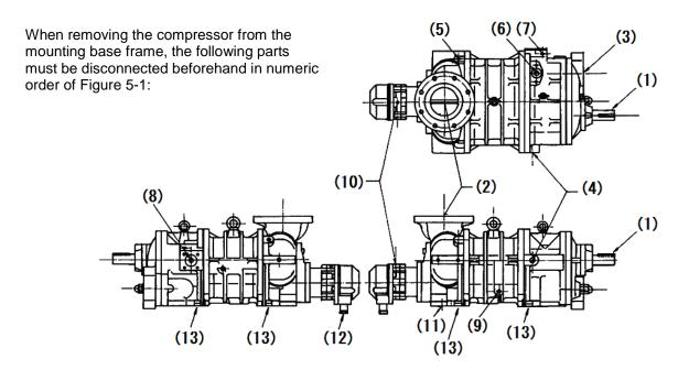
Figure 5-1 Disconnecting Parts
