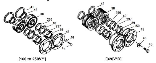
Figure 5-12 Exploded Views of Thrust Bearing Block
