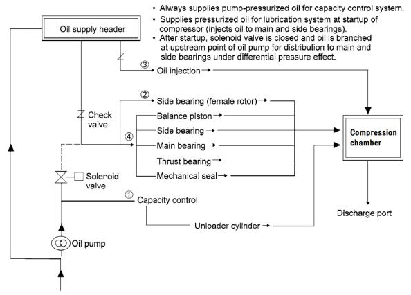
Figure 2-15 Oil Supply Route of Differential Pressure Oil Supply System
