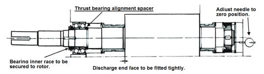
Figure 5-16 End Clearance Measurement Preparation
