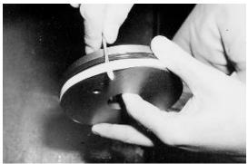
Removing the Cap Seal
