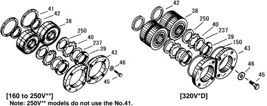
Figure 5-15 Exploded View of the Thrust Bearing Block
