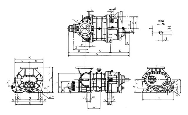
Figure 2-1 Outer Dimensions 160V\*D, 200V\*D, 250V\*D, 250VLLD (Sideways discharge type)
