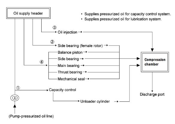
Figure 2-14 Oil Supply Route of Forced Oil Supply System
