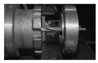
**Removing the Unloader Cover**
