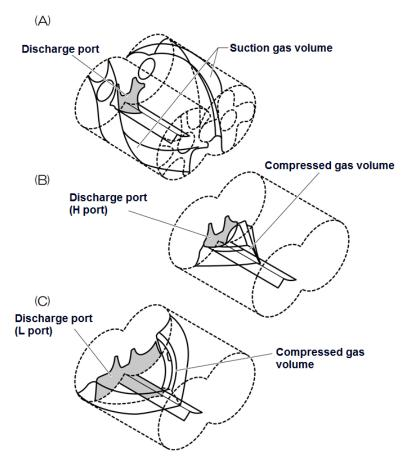
Figure 2-9 Internal Volume Ratio Vi
