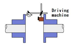
Figure 3-4 Measurement of Angularity
