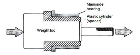
Figure 5-14 Example Tool for Press Fitting the Bearing
