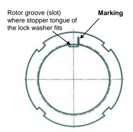
Figure 7-6 Position where mark is put
