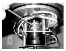
p) Turn counterclockwise until the micro switch lever is raised.
