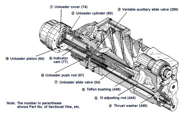
Figure 2-11 Variable Vi Mechanism of SCV-series
