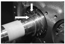
**Lock Washer and Torsional Slip Washer**
