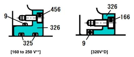
Figure 5-11 Difference around the O-ring gland
