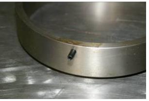
Type 2: Locked by a Spring Pin
