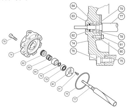
Figure 5-18 Unloader Cover Block
