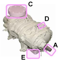
Figure 1-4 Hazardous Sources (Compressor: V\*G type)
