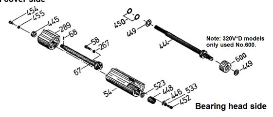
Figure 5-13 Variable Vi Auxiliary Slide Valve, Unloader Slide Valve and Vi Adjusting Rod
