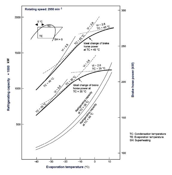
Figure 2-12 Refrigeration Capacity of Screw Compressor
