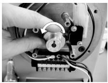
q) Slowly turn clockwise, and stop turning when the micro switch lever is lowered.
