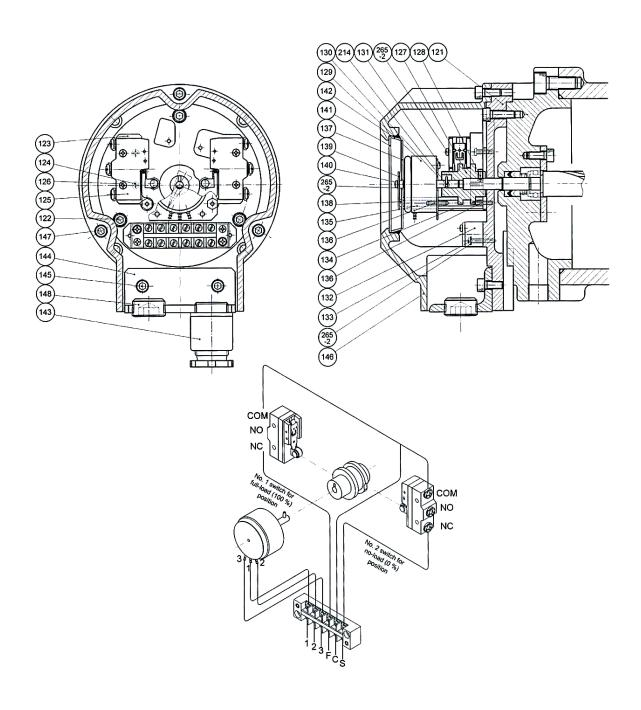
Figure 5-21 Sectional Views of SCV-series Unloader Indicator (Traditional standard type)
