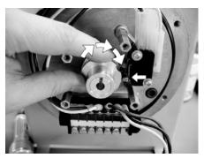
r) While holding the micro switch cam stationary, tighten the micro switch cam set screw.
