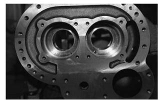
c) Install the O-ring [451] to the O-ring groove which located inside the hole to which is attached to the Vi adjusting rod of bearing head.
