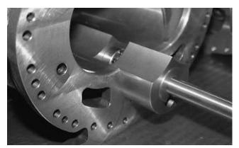
Pulling out the Unloader Slide Valve and Variable Auxiliary Slide Valve
