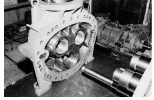
f) The O-ring and O-ring gland [326] are mounted in the unloader push rod passes part of the suction cover. Remove them. At this time, take care not to lose the four fastening screws for O-ring gland due to their smallness (M5). The structure and part No. of around the O-ring gland are slightly different between 320V\*D models and other models as shown in Figure 5-11.
