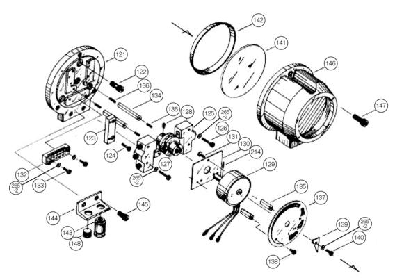
Figure 5-20 Exploded View of the Unloader Indicator (Traditional standard type)
