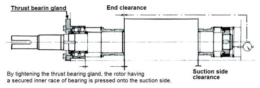
Figure 5-17 Measurement of the End Clearance
