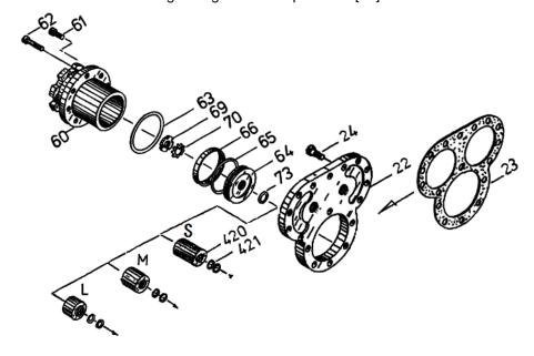
Figure 5-7 Unloader Cylinder Block and Balance Piston Cover (Example: 320V\*D)
