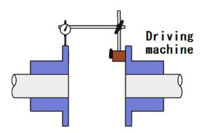
Figure 3-3 Measurement of Offset
