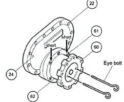
Figure 5-8 Removing the Unloader Piston
