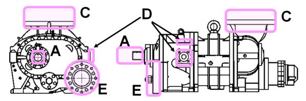
Figure 1-1 Hazardous Sources (Compressor: V\*D type i.e. discharge port facing sideways)
