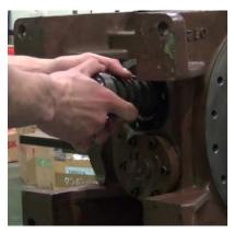
Photo 016 Removing Unloader Piston and Spring
