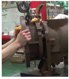
Photo 023 Installing Bearing Head
