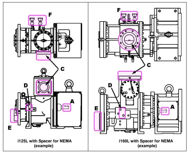
Figure 1-1 Locations of Hazardous sources (Compressor)
