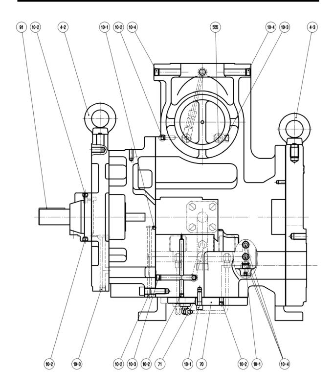
Figure 2-17 i160S Longitudinal Sectional View
