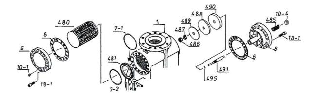
Figure 5-3 Suction Strainer and Check Valve (i160\*)
