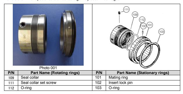
Figure 5-1 Details of BBSE Type Mechanical Seal Assembly
