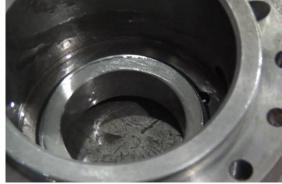
Photo 037 Tightening Seal Collar Set Screw
