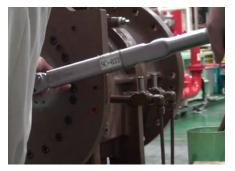
Photo 034 Final Tightening with Torque Wrench
