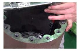
Photo 015 Removing i125-series Suction Adapter
