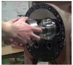
Photo 009 Removing the Balance Piston Sleeve
