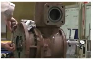
Photo 025 Tightening Thrust Bearing Gland
