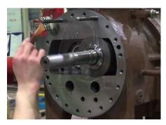
Photo 030 Applying Oil with Brush
