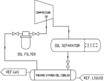
Figure app.1-3 is the reference flow of the thermo-siphon oil cooler.
