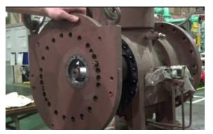
Photo 007 Removing Bearing Cover
