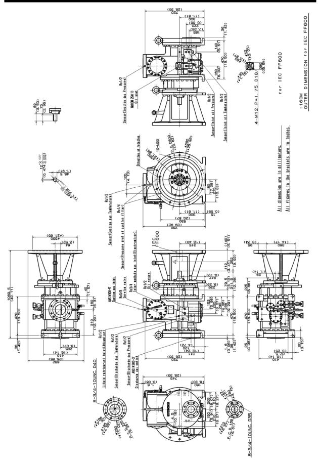
Figure 2-10 i160M Outer Dimensions with a Spacer for Flange Motor (IEC FF600)
