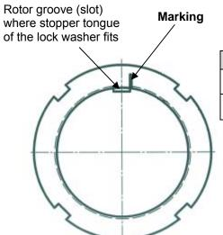
Figure 7-1 Position where Mark is Put
