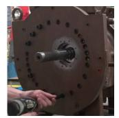
Photo 033 Temporarily Tightening Bolts
