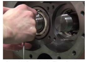
Photo 012 Removing the Thrust Bearing
