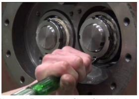
Photo 011 Extending the Claw of Lock Washer
