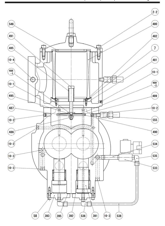
Figure 2-16 i125\* Longitudinal Sectional View of Suction/Capacity Control Section
