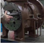
Photo 028 Installing Balance Piston Sleeve
