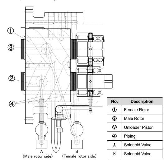
Figure 2-28 Capacity Control Mechanism
