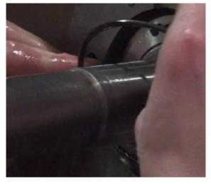
Photo 036 Inserting O-ring [49]
