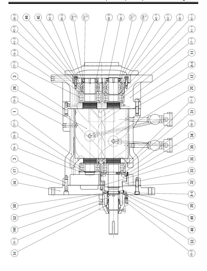
Figure 2-15 i125L Cross-Sectional View
