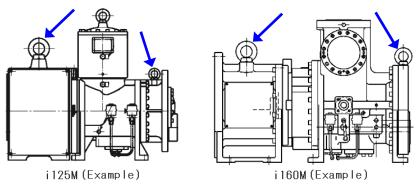
Figure 3-1 Eye bolts for lifting the compressor (Arrows)
