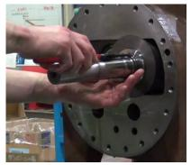
Photo 029 Installing Snap Ring
