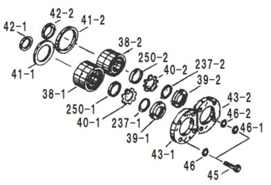
Figure 5-4 Thrust Bearings Block
