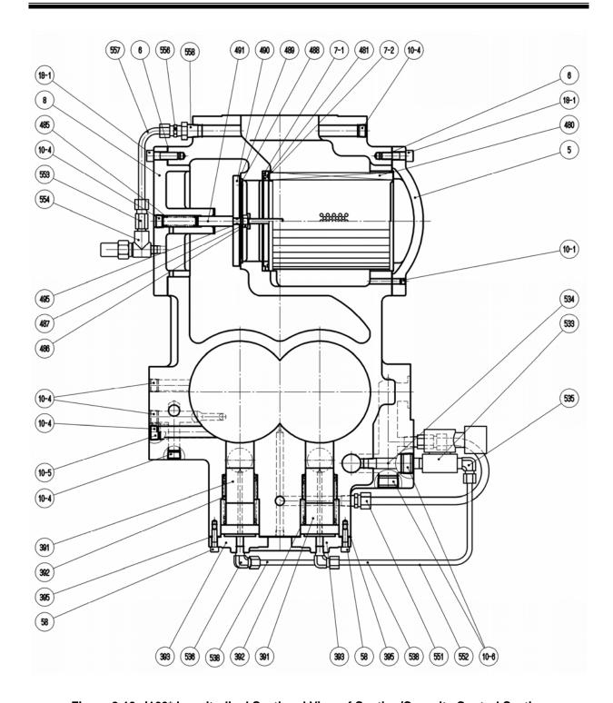
Figure 2-19 i160\* Longitudinal Sectional View of Suction/Capacity Control Section
