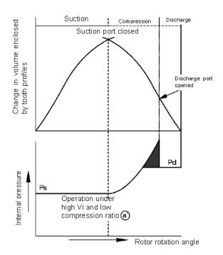
Figure 2-27 Relationship between Volume ratio (Vi) and Operation Conditions
