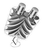
Figure 2-25 Discharge Process
