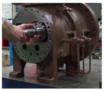
Photo 027 Installing Balance Piston
